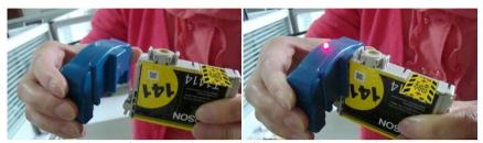
Press the terminals of the cartridge chip firmly against the pins on the resetter
