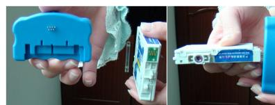
Press the terminals of the cartridge chip firmly against the pins on the
