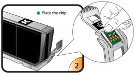
A dab of hot glue or instant glue may be needed to hold the chip in place. When using glue, be sure not to cover any contacts with it.
