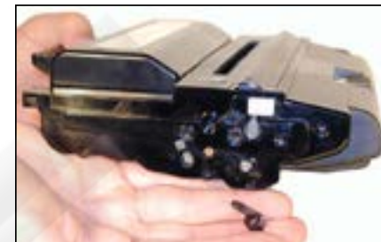
B.. Gently pry off the plastic drum axle bushing. Keep this bushing with the appropriate end cap when removed. Each side is different.
